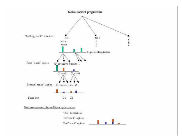
Figure 13: Illustration of the branch and bound method.
