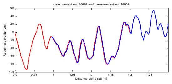
Figure 32: Result of automatic least squares fitting after manual shifting.
