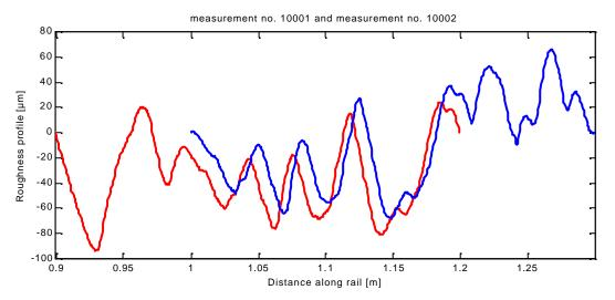
Figure 31: Fitting procedure. At start, data is displayed assuming exactly 20 cm overlap.
