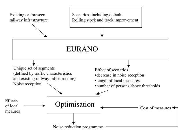
Figure 14: Process diagram showing interaction of optimisation with Eurano.
