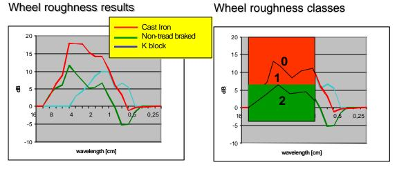
Figure 38: Example of Wheel Roughness Classification
