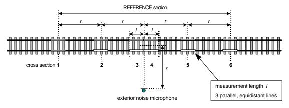
Figure 27: Measurement map for rail roughness
