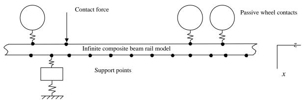
Figure 21. Diagram of the new track model, 'cobra'.
