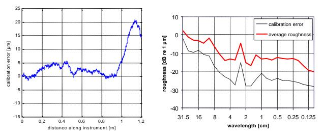
Figure 36: Left: estimated calibration error or error profile. Right: spectrum of 4 concatenated error profiles.
