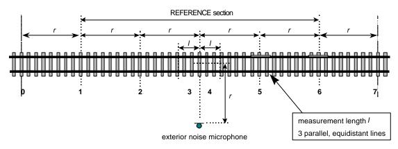
Figure 29: ISO procedure, with extended sections 0 and 7.
